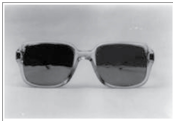
Figure 5. A specially constructed bifiltered spectacle with red and green glasses on the top halves and crossed polaroid filters on the lower halves
